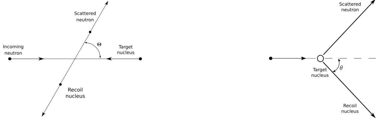
Figure 3.3: Diagrams illustrating the lab frame (left) and center-of-mass frame (right) of a neutron scattering elastically with a target nucleus.
