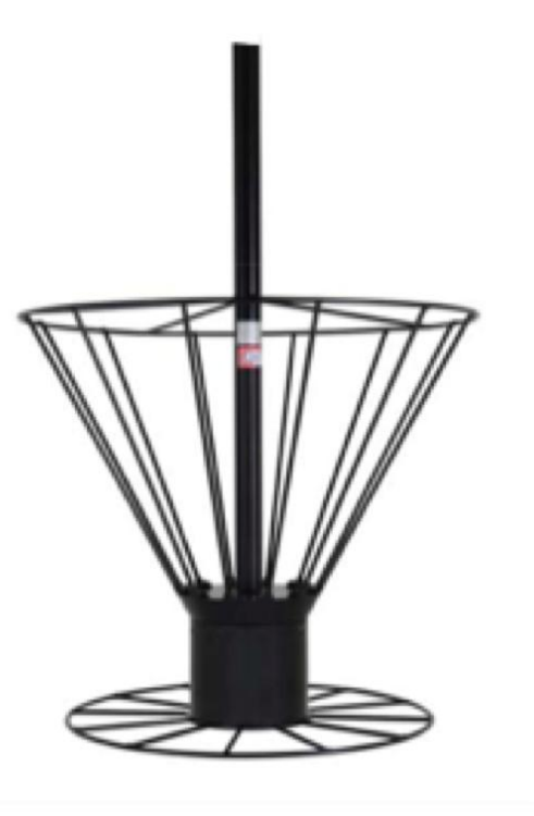
Figure 3.14: Images of the calibration pulser antennas deployed at WAIS divide and Siple Dome for calibration of the ANITAIII instrument in flight. Right: Custom designed, quad-slot "Mini-ALFA" antenna for horizontally polarized signals. Left: a Telewave ANT280S discone vertically polarized antenna. [10]
