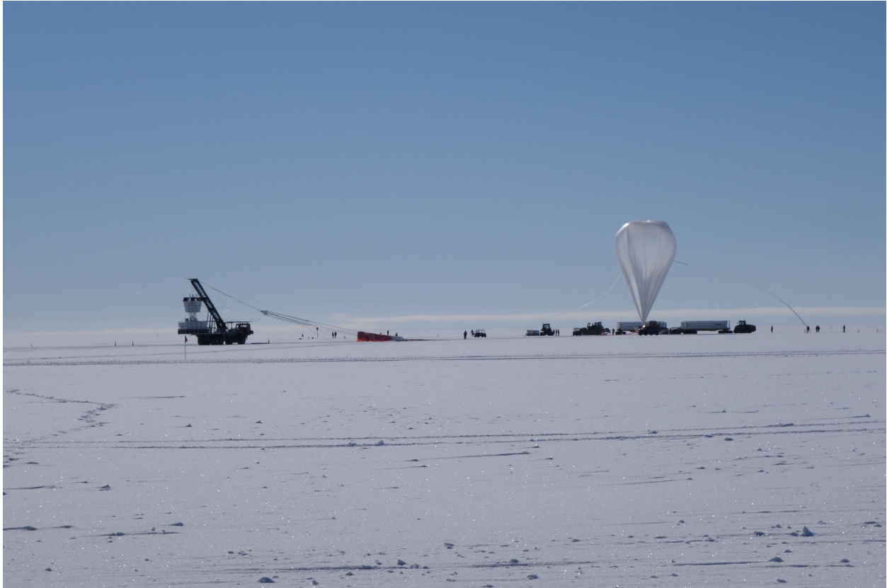
Figure 2.27: Image of the launch vehicles, the balloon, and the ANITA-III instrument immediately preceding launch on December 17th, 2013. On the left of the image is the LDB launch vehicle, named The BOSS, suspending ANITA. Attached to ANITA and the launch vehicle laying across the ice is the termination package, including a parachute for decent, and balloon. The tanks in the background are transportation canisters for the Helium gas, which is filling the balloon through the transparent hoses attached on the sides.
