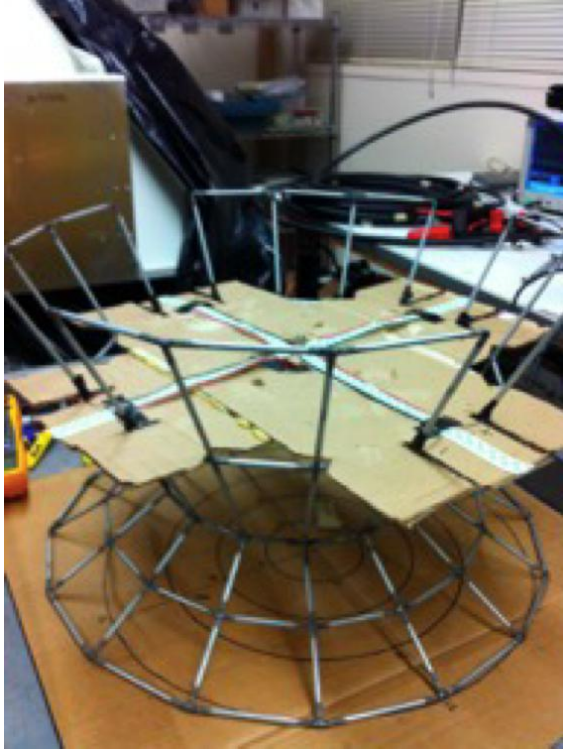
Figure 3.14: Images of the calibration pulser antennas deployed at WAIS divide and Siple Dome for calibration of the ANITAIII instrument in flight. Right: Custom designed, quad-slot "Mini-ALFA" antenna for horizontally polarized signals. Left: a Telewave ANT280S discone vertically polarized antenna. [10]
