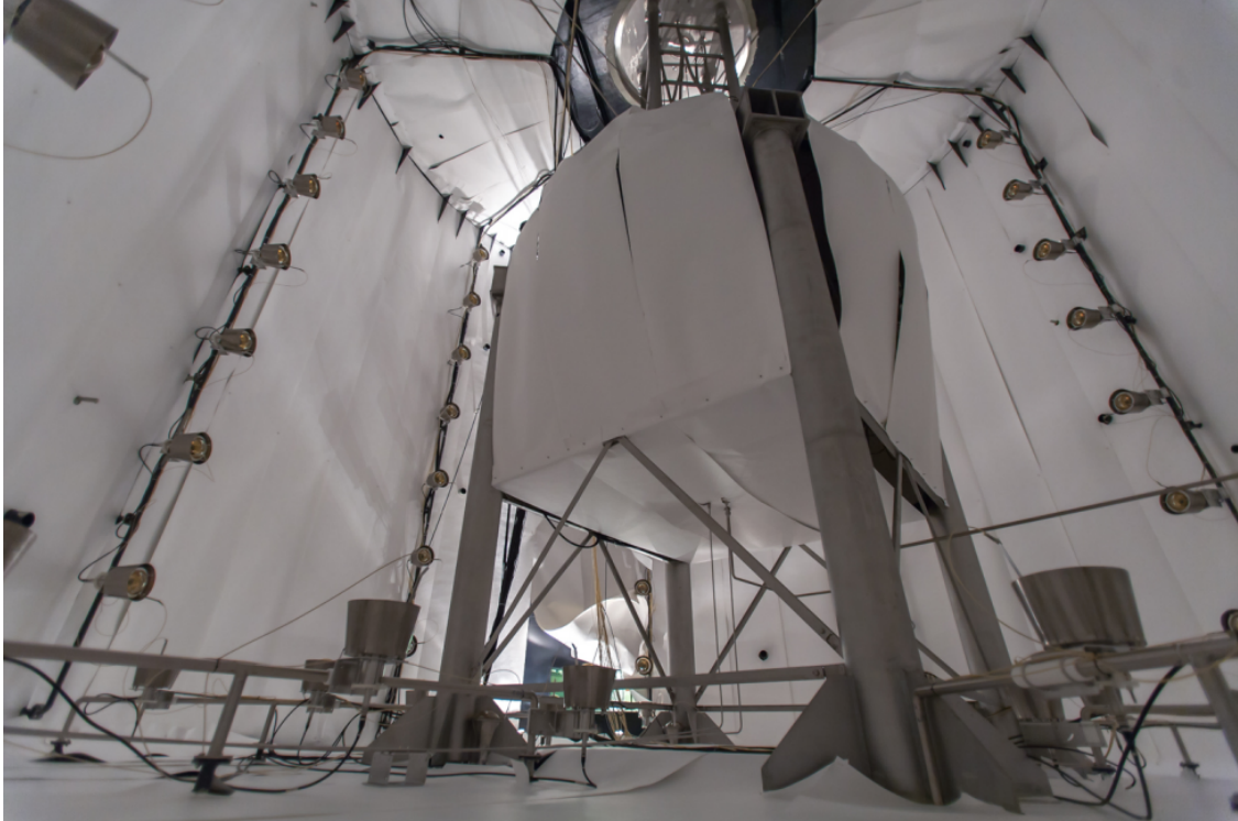
Figure 3.7: Photograph of the interior of the WCV, prior to being filled with ultra pure water. The LSV is in the center. All surfaces are covered with highly reflective Limirror.
