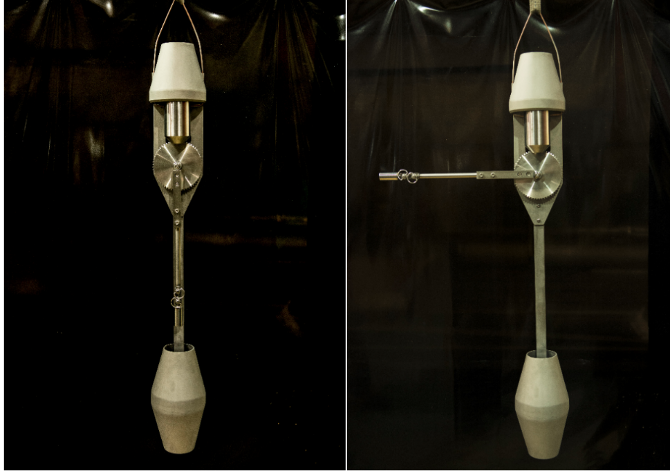
Figure 4.4: The source deployment system, called the PIG, with the source arm vertical (left) and articulated to horizontal (right). The source arm showed in this picture is 40.31 cm, however the arm used in deployments is 62.0 cm in order to put the source holder in contact with the cryostat.
