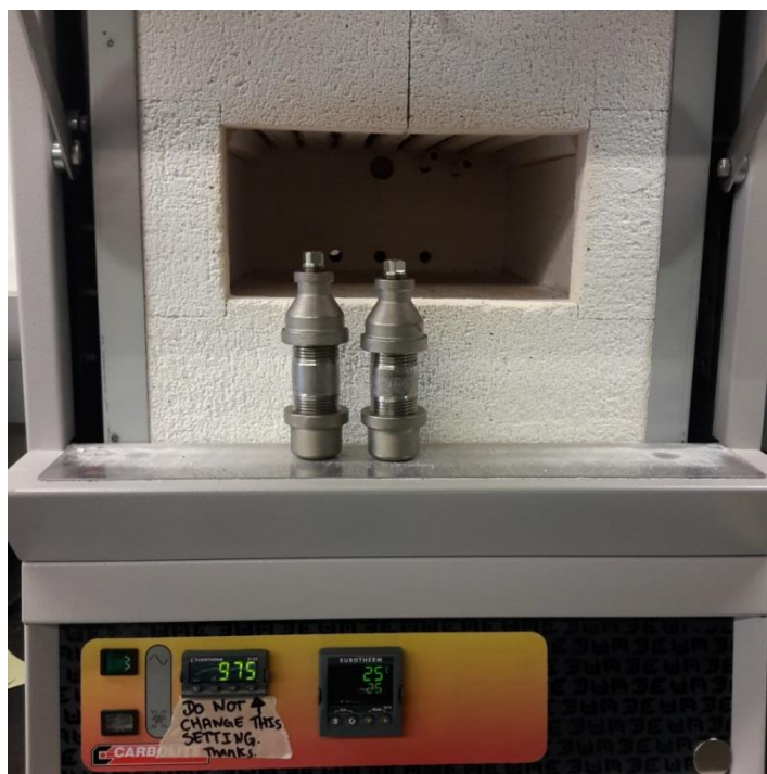
Figure B.6. Torrefaction reactors
