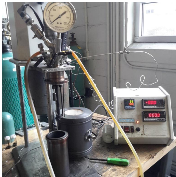
Figure B.8. Hydrothermal carbonization reactor
