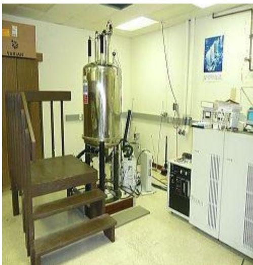
Figure 22: A 500 MHz NMR spectrometer used at the University of Hawaii at Manoa. Photo courtesy of the UH Manoa Chemistry website.
