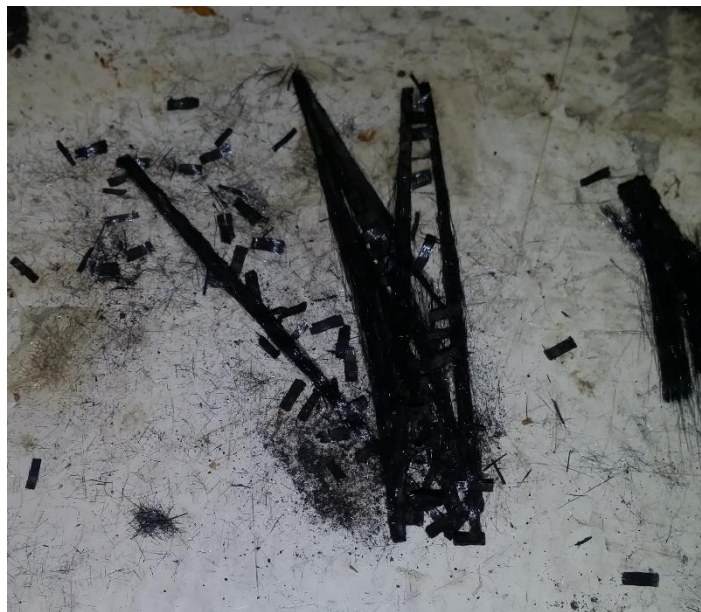
Figure 3.10: Carbothermal decomposition of Nicalon™ laminates at 1500°C PIP.
