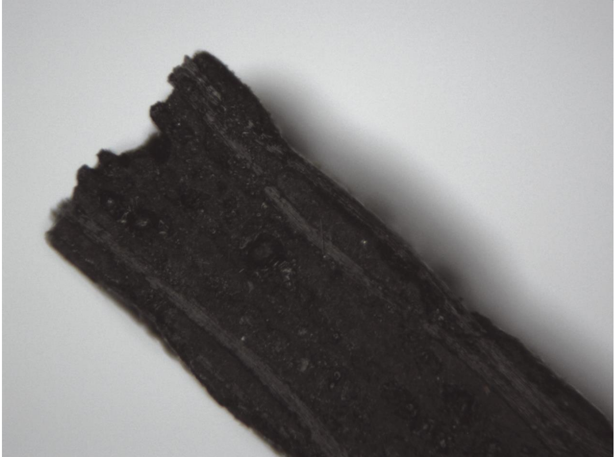
Figure 5.7: Optical micrograph of T300 CFCC mid-span failure.
