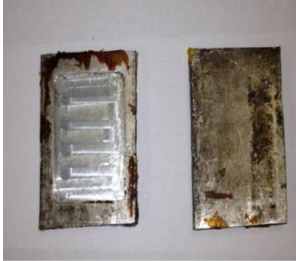
Figure 3.1: Manufactured Aluminum mold.
