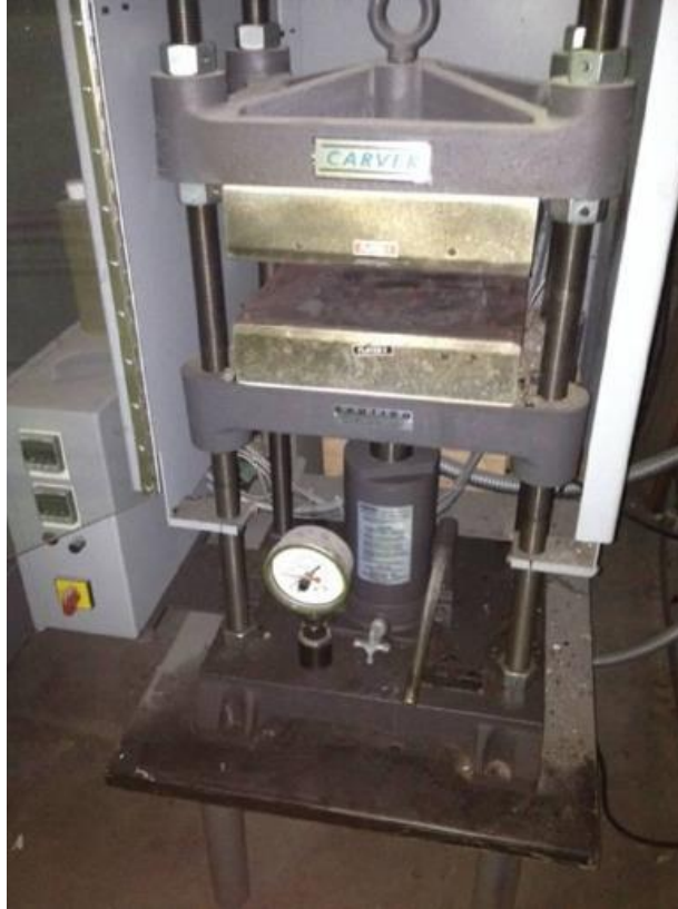
Figure 3.2: Compression molding machine.
