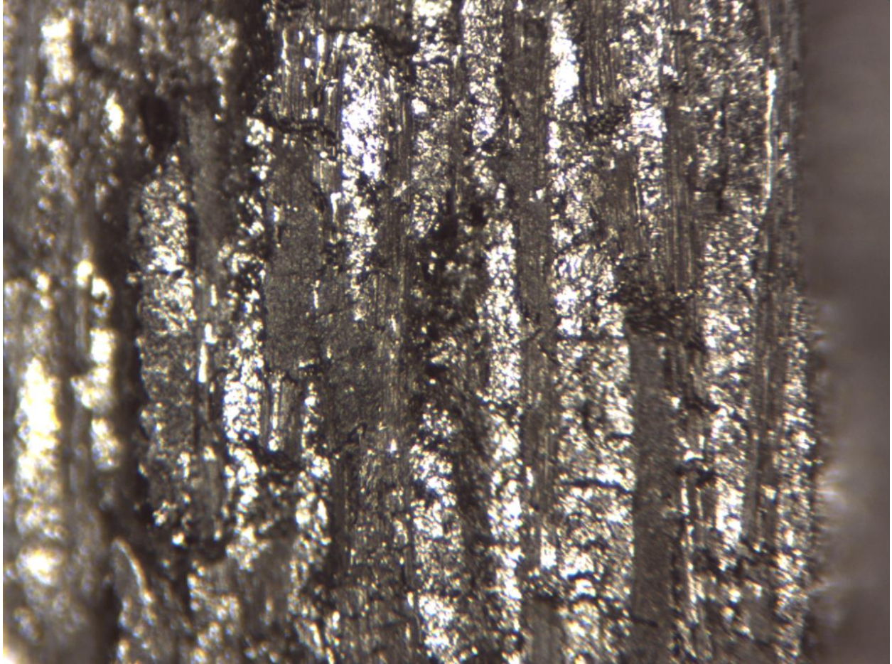
Figure 5.44: Typical fracture surface of 1500°C pyrolyzed CFCCs showing a brittle fracture.
