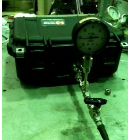
Figure 3.9: Modified Pelican® case used as a vacuum compartment [37].
