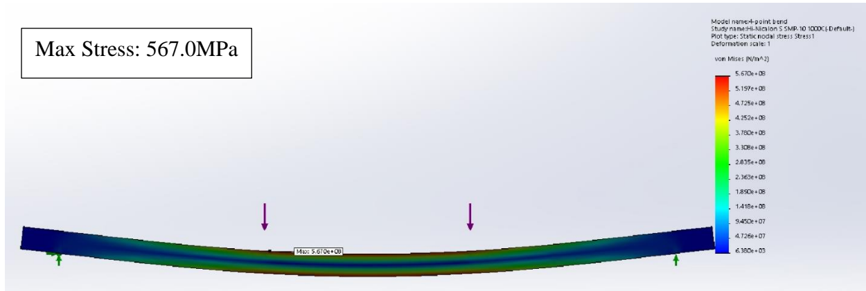
Figure 5.69: Stress simulation for Hi-Nicalon™ Type S SMP-10 CFCCs pyrolyzed at 1000°C.
