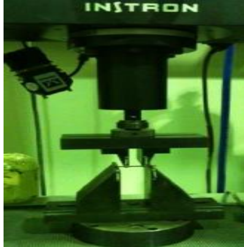
Figure 5.3: Four-point bending test fixture.
