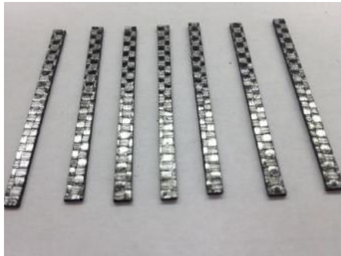
Figure 3.5: Cured and cut green ceramic composite beams.
