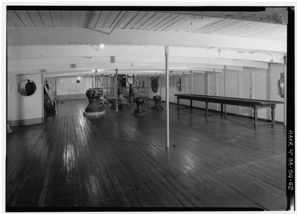
Figure 9 – View of shelter deck with original decking. The ceiling here was added later in Balclutha ’s history when the poop deck above was extended and this space was used for more cabins. 138
