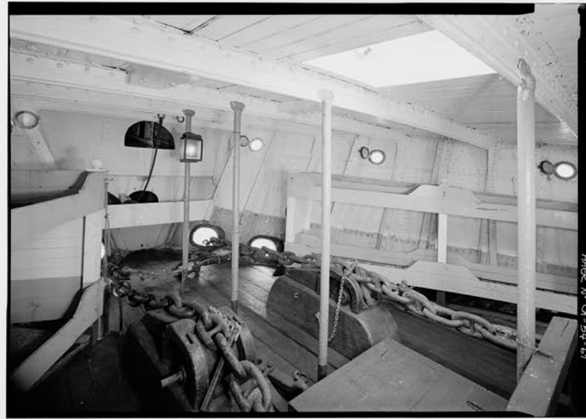
Figure 6 - View of the fo'c'sle from port side. Bunks are wood with little personal space. Anchor chains and hawse pipes as from description above are visible. 112
