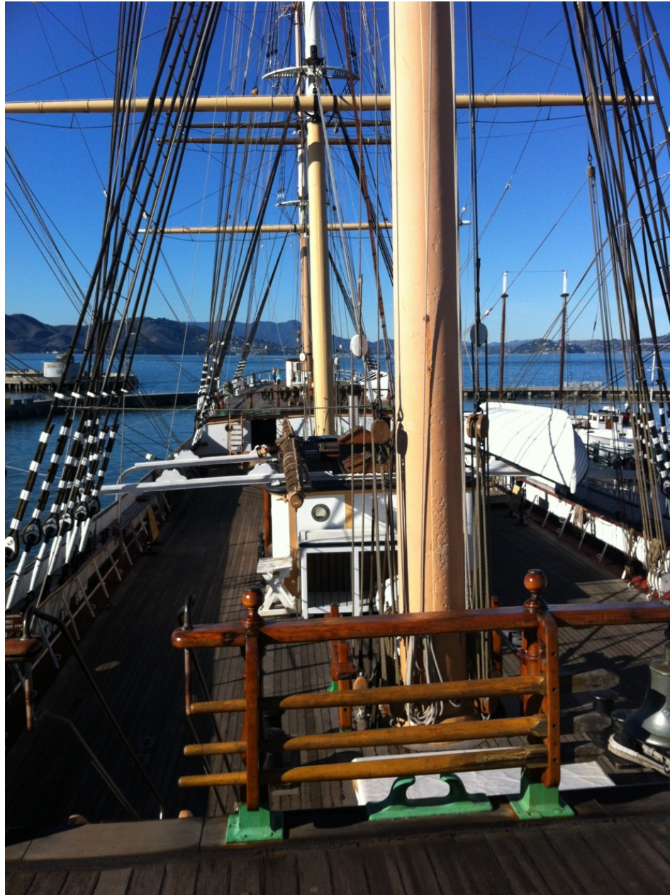
Figure 10 – View from Balclutha 's foredeck, directly above the fo'c'sle, looking toward the stern. The foredeck rails are clearly visible in the foreground, but there are also rails visible on either side of the main deck near the hull. On the starboard side, left in the image, is the ladder leading down from the foredeck to the main deck. In the middle of the image, just aft of the foremast, is the deckhouse with an animal pin in front. All of these items were mentioned in the sources as having been made, or partly made, of teak. Photo taken by author, February 2016.
