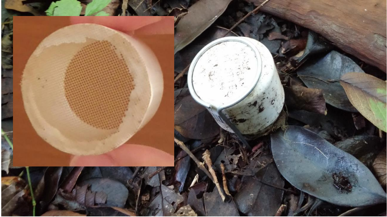
Figure 2.2. Amdro bait station design. Stations were constructed of PVC piping with removable endcap tops and glued screened bottoms, and staked to the ground. This facilitated easy bait replacement and allowed for ants to access the baits.
