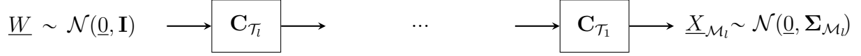
Figure 4.2b: The l stages of model approximation using cascade tree transformation decomposition framework. The model approximation is generated by passing \underline{W} \sim \mathcal{N}(\underline{0}, \mathbf{I}) through the l steps of cascade trees and is \underline{X}_{\mathcal{M}_l} \sim \mathcal{N}(\underline{0}, \underline{\Sigma}_{\mathcal{M}_l}) .
