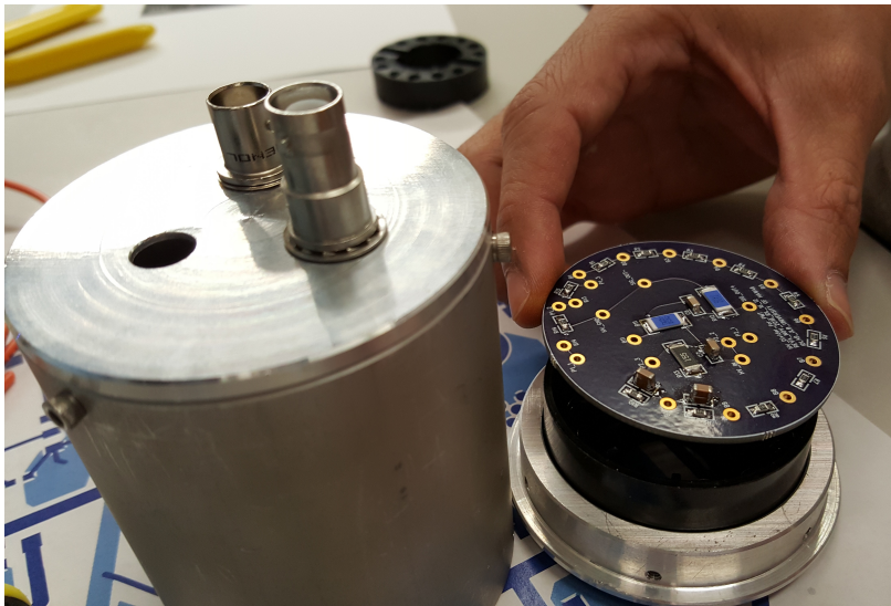
Figure 2.11: HV base enclosure (left) Internal HV divider board assembly (right).
