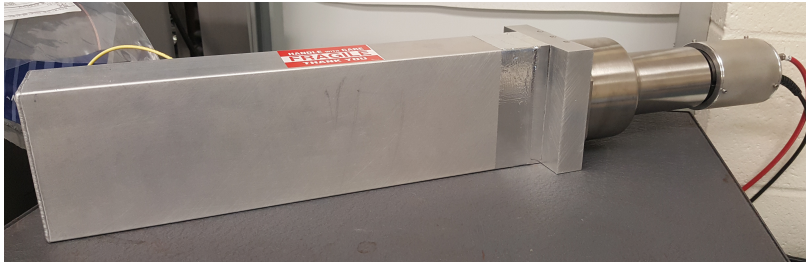
Figure 2.6: Square cross-section NaI scintillation detectors.
