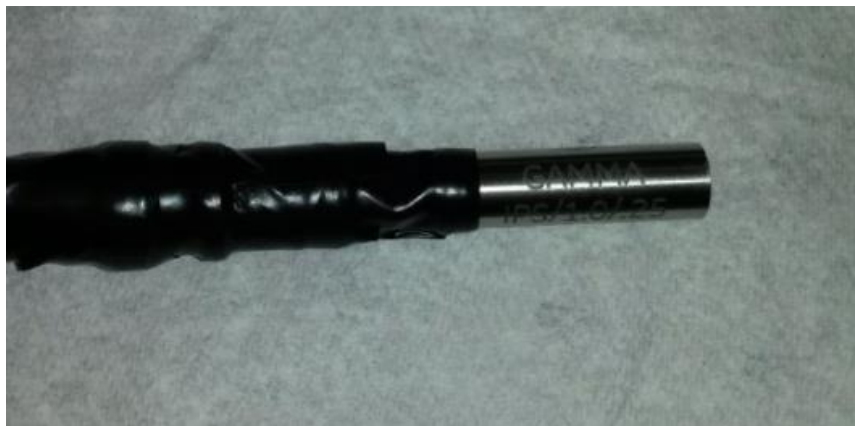
Figure 2.4: An ultrasound transducer manufactured by General Electric (GE). This transducer has a 6.35-mm-diameter face, and is approximately 76.2 mm long. The black tape on this transducer is to prevent any water leakage during the ultrasound characterization process.
