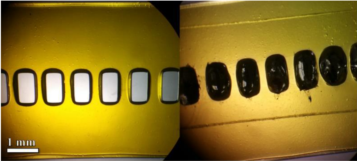
Figure 3.11 Images of TMPTA microstructures fabricated for TLM experiment before (left) and after (right) Galinstan Injection.
