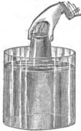
Figure 12. Simple Experiment for Students to Conduct, Demonstrating Atmospheric Pressure (Gage, 1882, p. 2)
