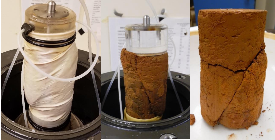
FIGURE 5.21 Photos of sheared specimen from tests (a) CWCU-1, (b) CWCU-2, and (c) CWCU-3
