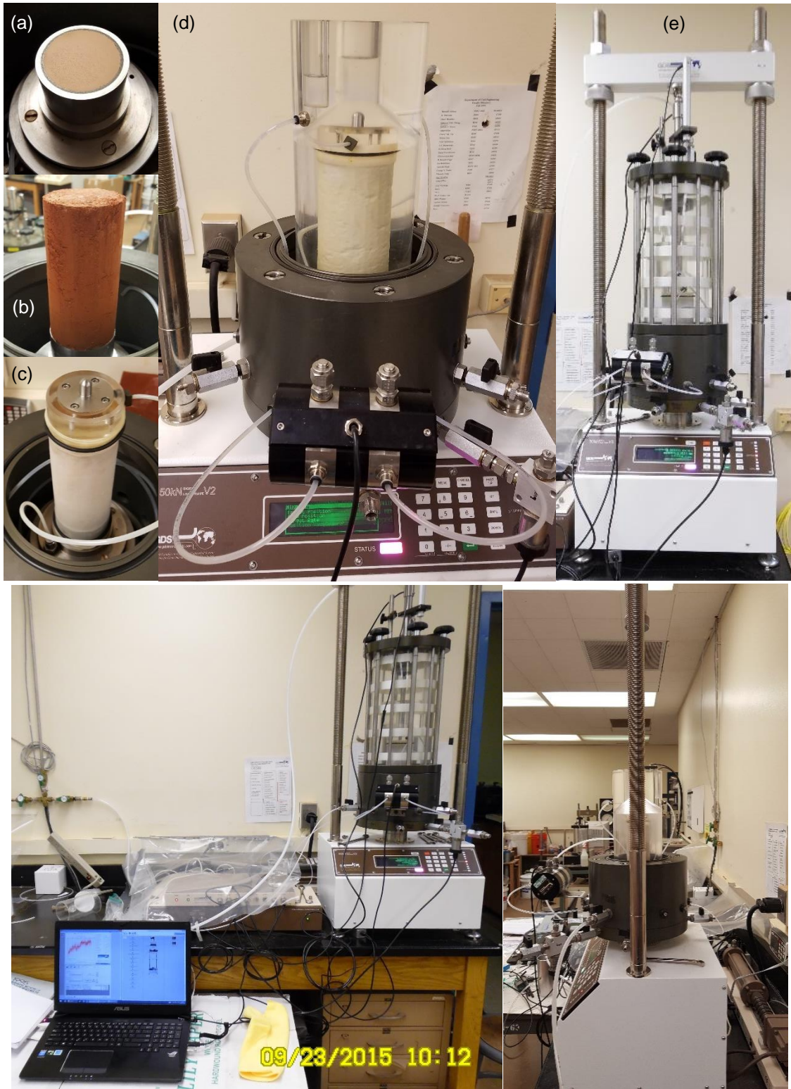
FIGURE 5.20 GDS triaxial apparatus with HKUST double wall volume change measurement system
