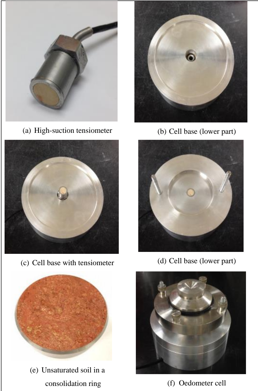
Figure 2.3 Assembly for one-dimensional oedometer compression test
