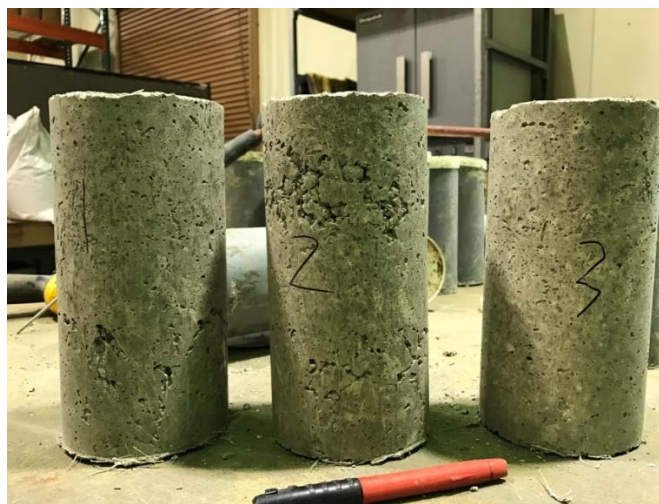
Figure 6-7 Severe honeycombs of 4"x8" cylinders due to fast drop in workability
