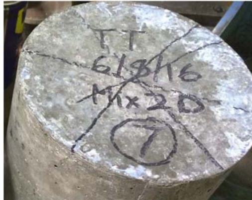
Figure 6-1 Latex bleeding as concrete hardened
