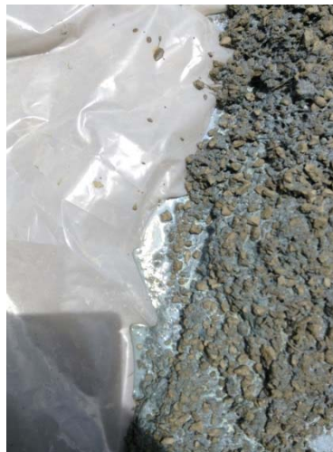
Figure 4-6 Bleeding mix using Type I/II cement in place of Rapid Set cement
