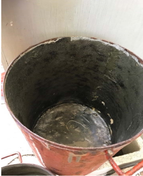
Figure 4-4 Epoxy-coated drum for fibers collection
