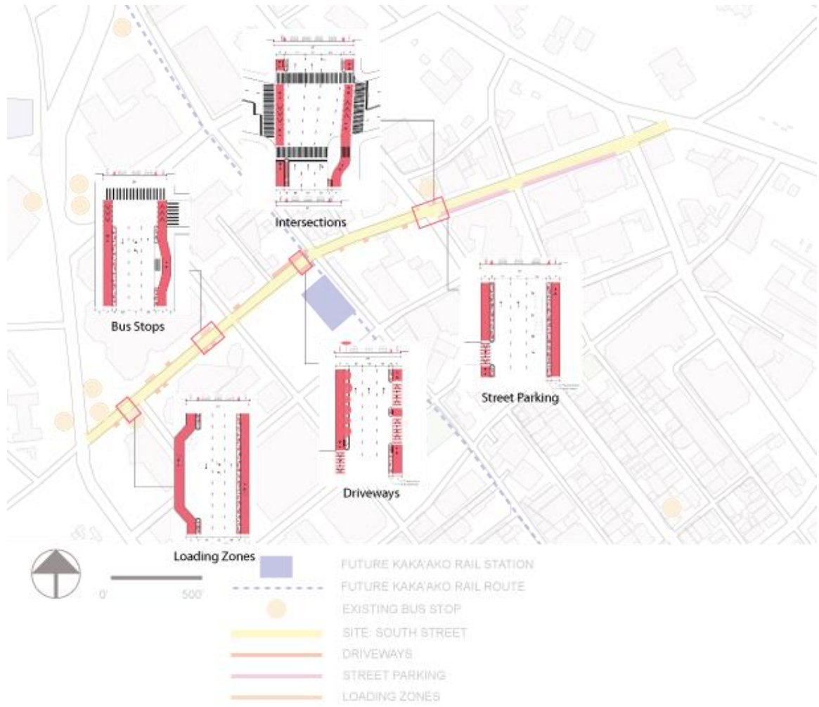
Figure 87: Conflicts and Resolutions Using Bike Facility Design. Graphic by: Author.
