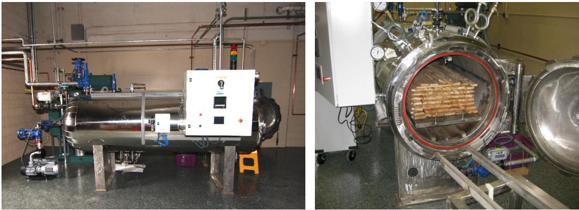
Figure 8.40: Thermal Modification Kiln at the Natural Resources Research Institute
