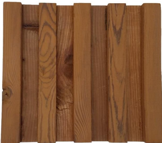
Figure 8.48: Thermally Modified Brettstapel (Elevation View)
