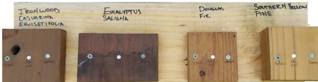
Figure 8.46: Fastening systems in thermally modified timber
