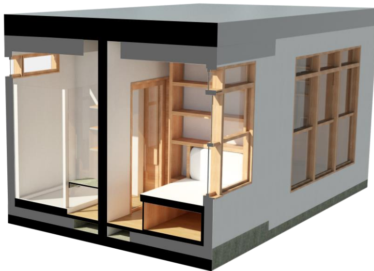
Figure 52 Section Perspective Through Sub-Volumes to See How They Fit Inside for Transportation
