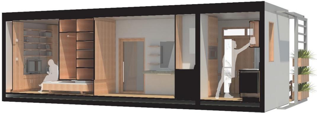
Figure 50 Section Perspective Through Sub-Volumes to See How They Fit Inside Unit for Transportation
