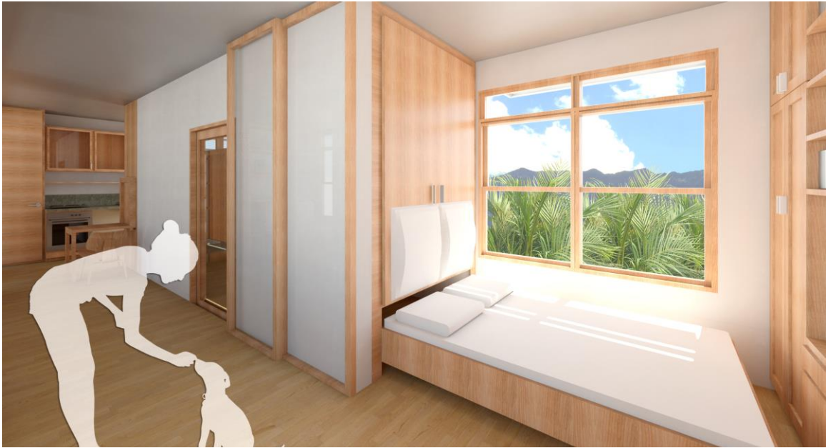
Figure 53 Interior Rendering of Unit from Bedroom: Shows the Bed Pulled-out and Rotating Wall Open
