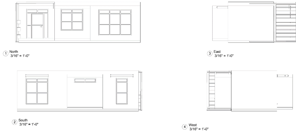
Figure 47 Accessory Dwelling Unit Elevations
