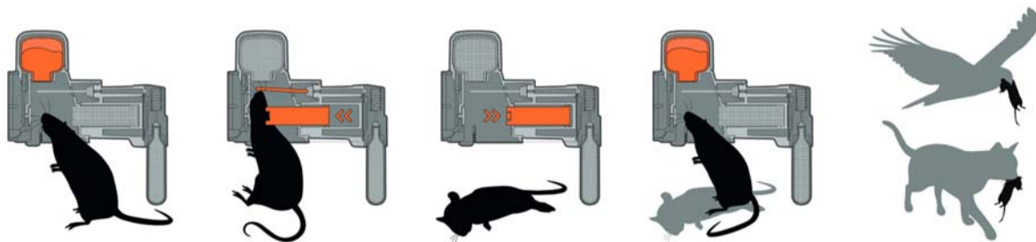
Figure 3: A24 Trap function Lure attracts rats to trap; trap fires when trigger is brushed; trap clears and automatically resets after a humane kill; trap can attract and dispatch up to 23 additional rodents before needing service; carcasses are often scavenged from below the trap. Image courtesy of Goodnature®
