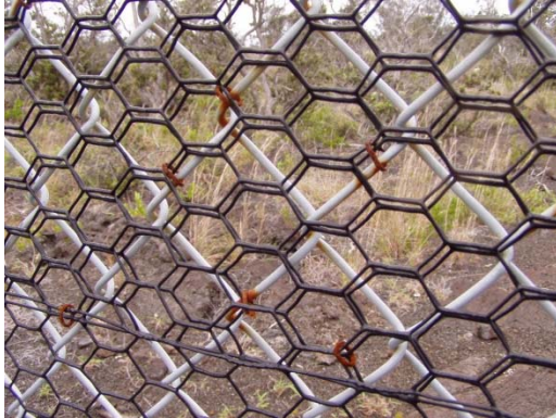
Figure 9 Non-galvanized hog rings after one year
