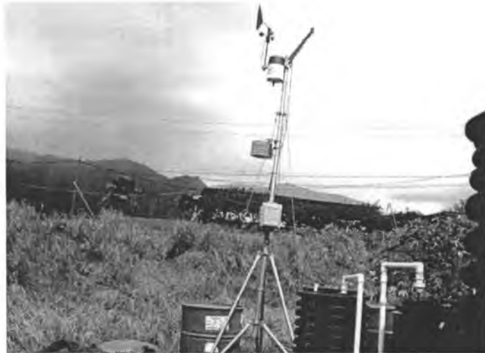
Plate 3.6. A portable weather station was installed at the site to monitor various climatic data.
