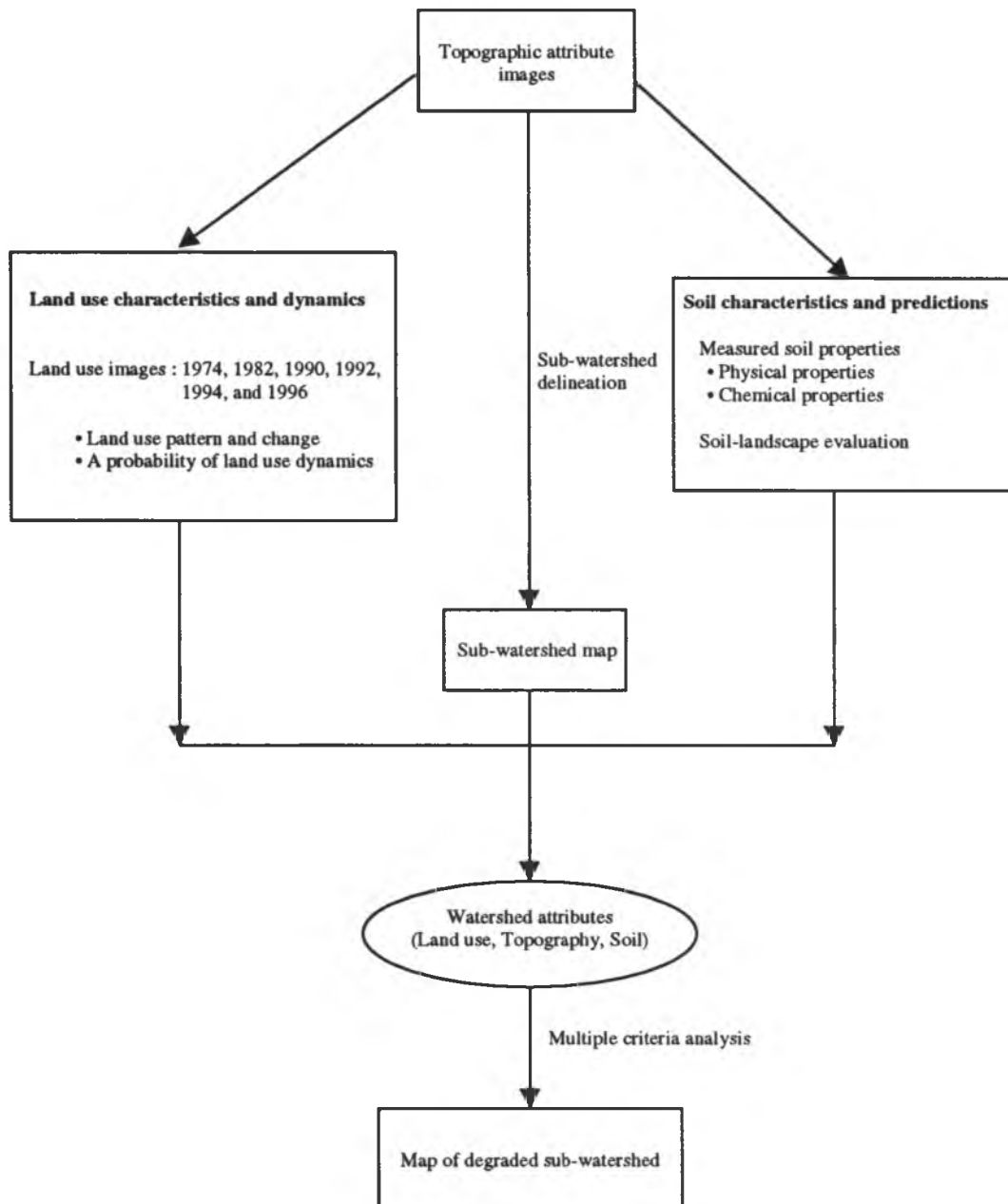
Figure 1.1 A framework for using landscape characteristics and dynamics to improve management of the Wat Chan watershed, Thailand.
