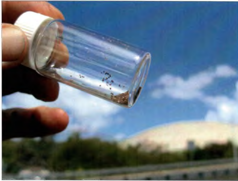
Figure 2.2. The amount of seed used in the hydroseeding treatment. The vial contains 0.1 grams or approximately 1500 seeds.
