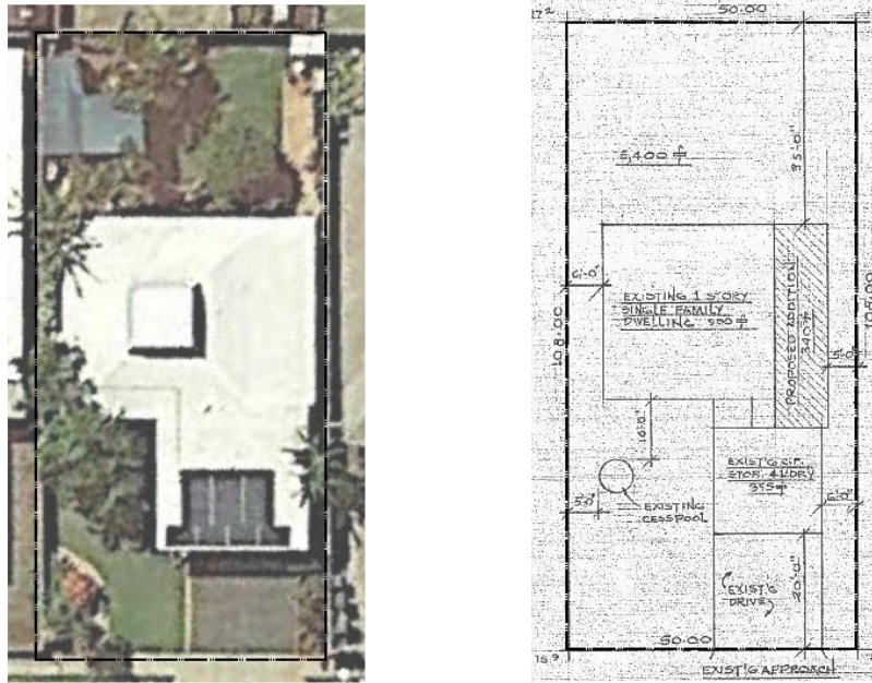
Figure 7.3– A map depicting the aerial satellite view and Tax Map Key (TMK) site plan of the example property to be designed. (Left Image Source: Google earth)
