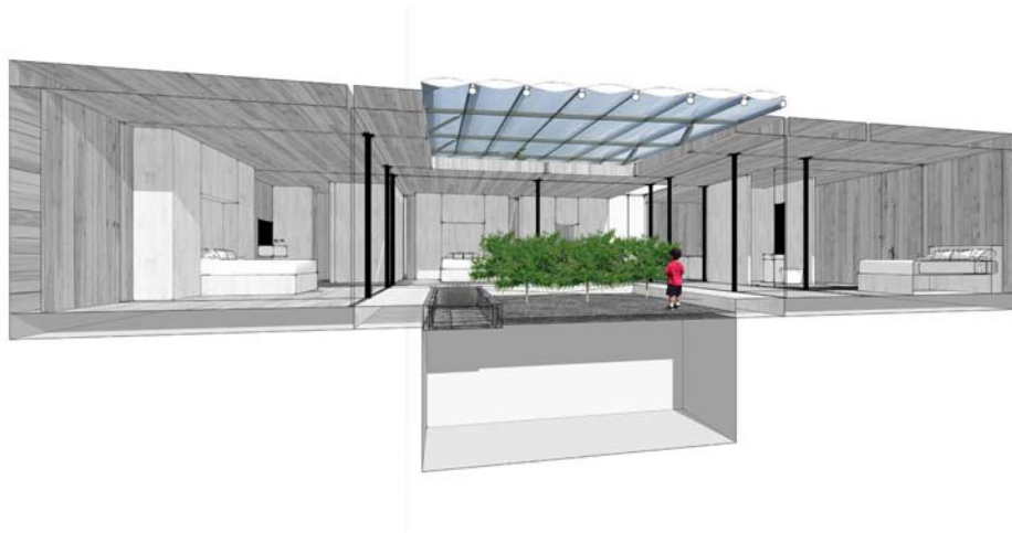
Figure7.7 Movable ETFE on courtyard (winter)
