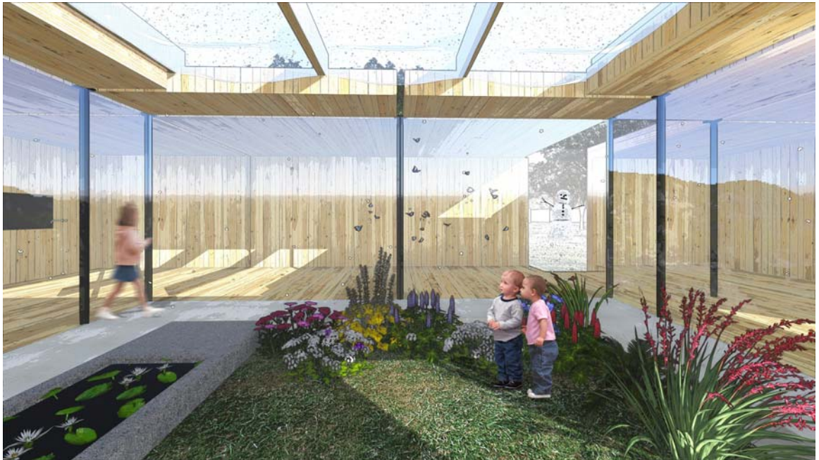
Figure 5.11 Courtyard with ETFE roof in winter
