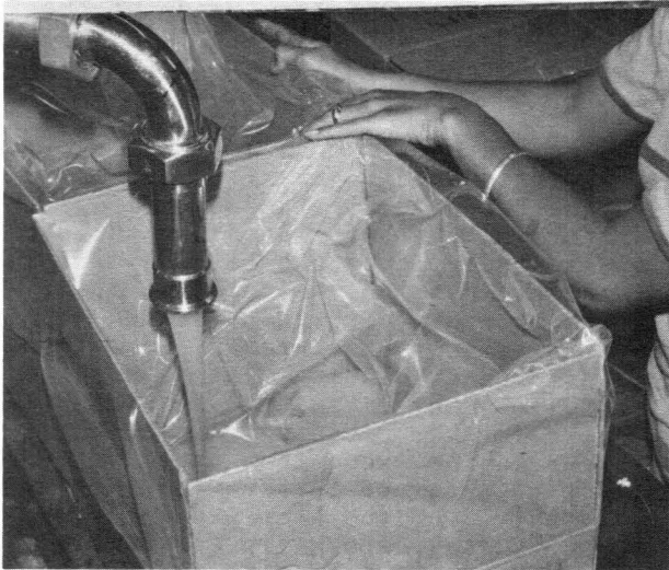
Figure 13. Filling puree into plastic-lined cartons
