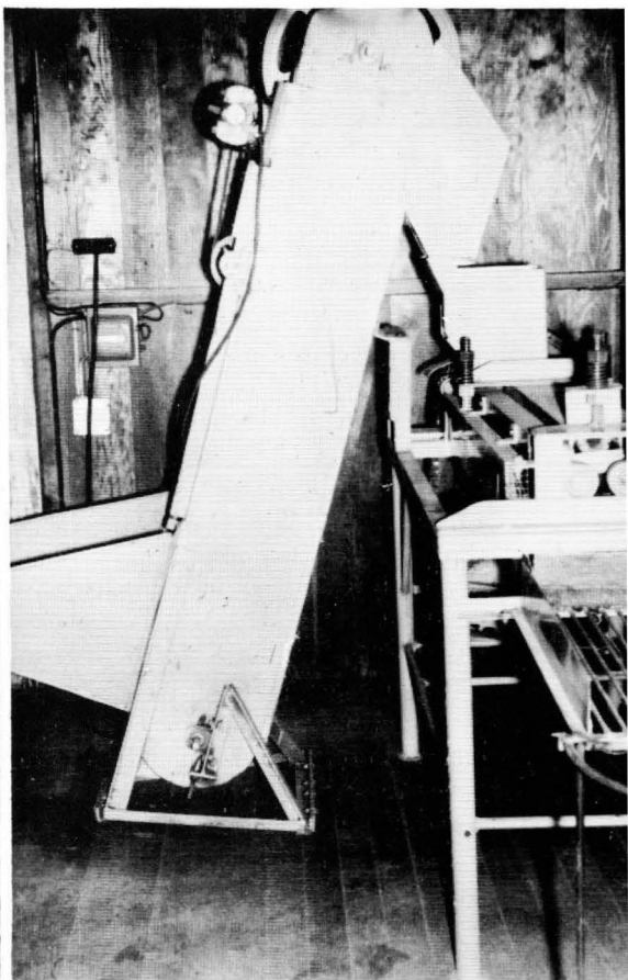
Bin, elevator, and screw type husker currently being used in processing macadamia nuts.
