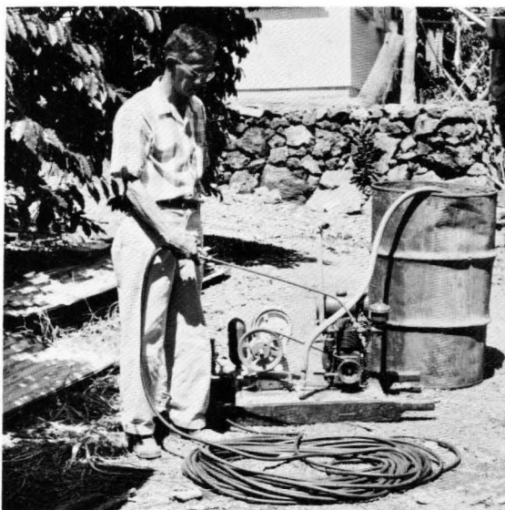
This two-man power sprayer is used in conjunction with 55-gallon drums spaced throughout the orchard.
