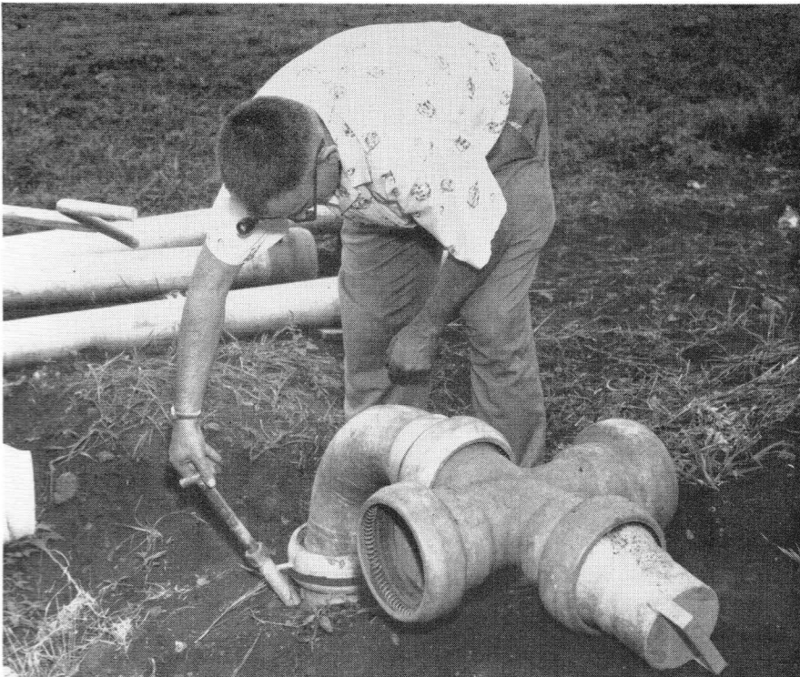
Fig. 32. Outflow from a metal riser is controlled by turning the valve handle. The elbow outlet can be adjusted to any desired direction. The hydrant can be provided with multiple outlets.
