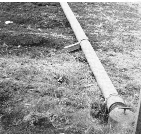
Fig. 29 (right). A lightweight hydrant, open at the top, is placed over alfalfa or orchard valves where low heads are assured. It allows surface discharge and conveyance to distant furrows by additional surface pipe. Outflow from the hydrant into either surface pipe is controlled by a sliding gate.
