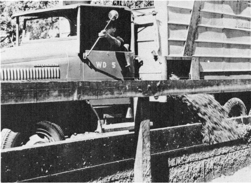
Fig. 18 – Kekaha Sugar Company Ltd. self-unloading truck unit (see also Figure 17) dispensing greenchop alfalfa into feed bunks at Meadow Gold Dairy, Waimea, Kauai. Such trucks can save much time and labor in a well-planned greenchop production system.
