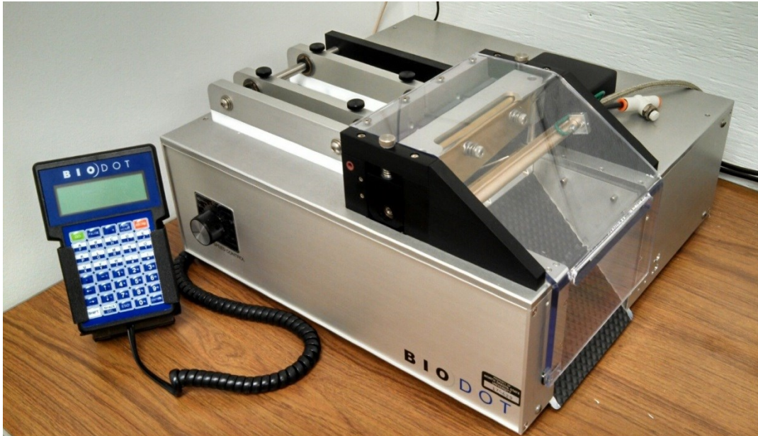
Figure 4: Image of a fully automatic workstation, Guillotine cutting module CM 4000 that uses data input to cut biosensor to a desired width and speed, providing high-quality precision cuts.
