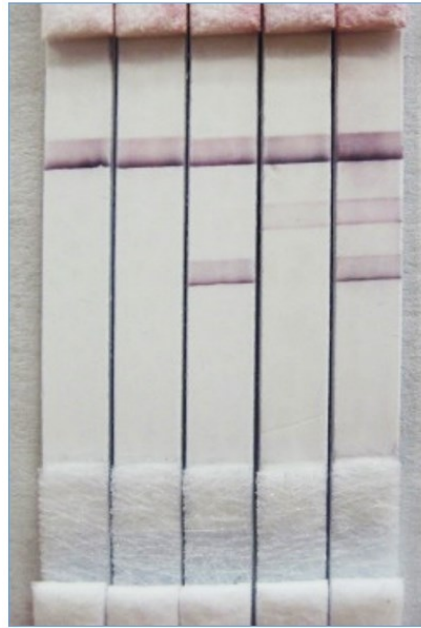
Figure 37: Typical photo images of (1) and (2) represent control conditions with 10 \mu l NTC + 90 \mu l Water. (3) and (4) show the presence of 10 \mu l NG target and CT target respectively. Strip (5) is the presence of both targets in equal volumes. Assay time: 20 minutes
