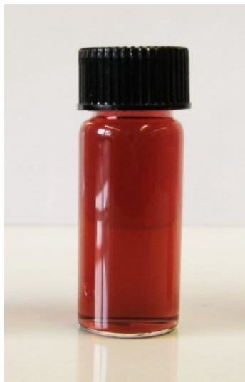
Figure 1: Image of 15 nm sized colloidal gold nanoparticle prepared using citrate reduction method.
