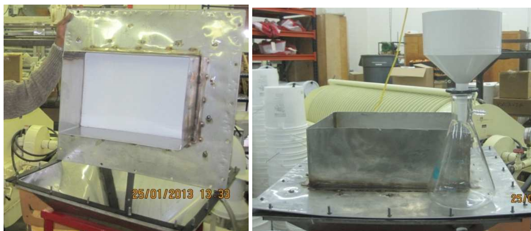
Fig. C1: Pictures of the separatory funnel used as a washing and a filtration unit
