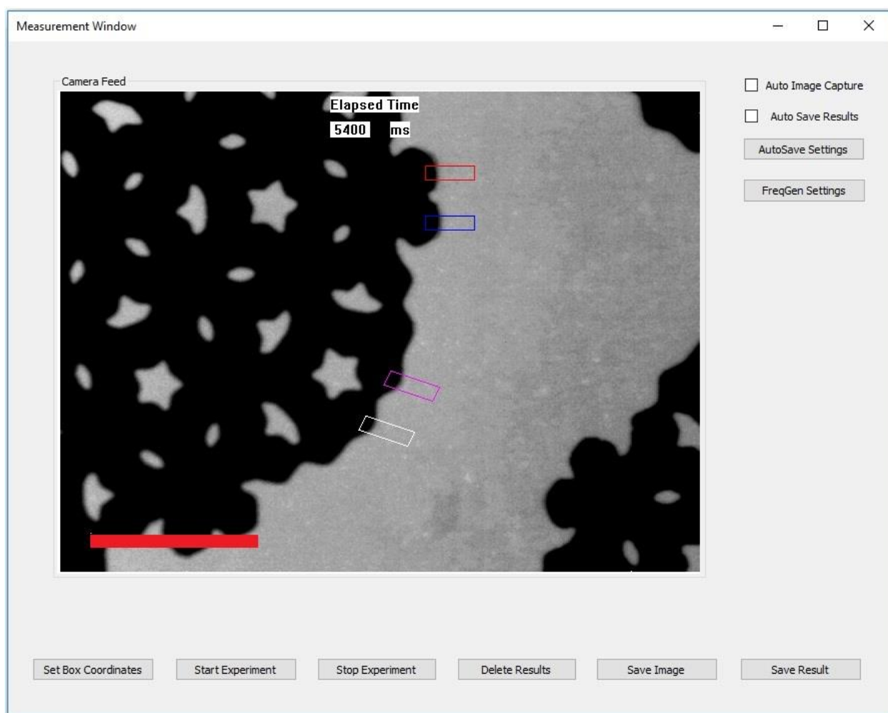
Fig. 20. Microsoft Windows application for DEP Spectroscopy. The regions of interest are marked with colored rectangles. PID electrode is visible as darker region in the picture. Scale bar indicates 100\ \mu\text{m} . 52
