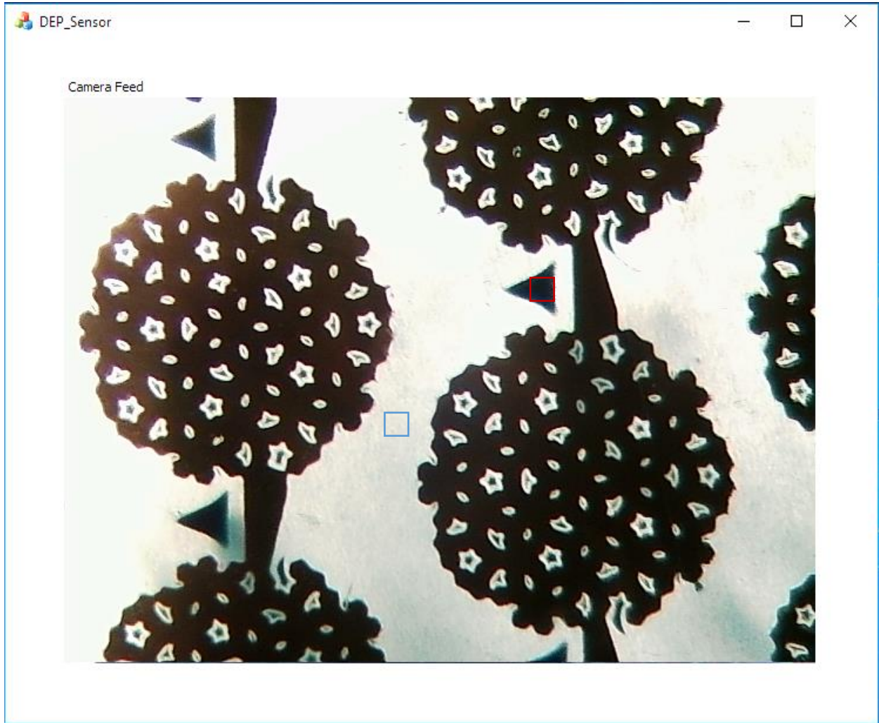
Fig. 13. The camera feed in DEP spectroscopy application with regions of interest marked by red (for negative dielectrophoresis) and blue (for positive dielectrophoresis) rectangles 51
