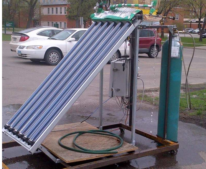
Figure 26: Evacuated tube U-pipe solar collector used for experimental set-up
