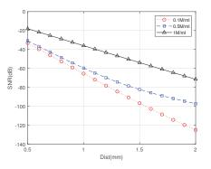
Figure 4: SNR versus path length in dermal equivalent with three cell densities using Gaussian-shaped power distribution.
