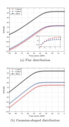
Figure 3: SNR versus transmitted signal power for THz communication inside artificial skin using (a) flat and (b) Gaussian-shaped distribution, and the communication distance is 1 mm.
