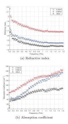
Figure 2: Frequency-dependent refractive index and absorption coefficient of dermal equivalent with three different cell densities, namely, 0.1 M/ml, 0.5 M/ml and 1 M/ml.
