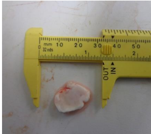
Figure 4. Cross sectional brainstem tissue sample prepared for compression tests
