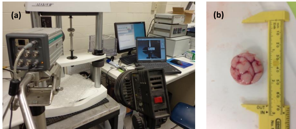
Figure 3. Sample preparation and experimental setup (a) the Electroforce machine (b) a cylindrical brain tissue sample for a compression test
