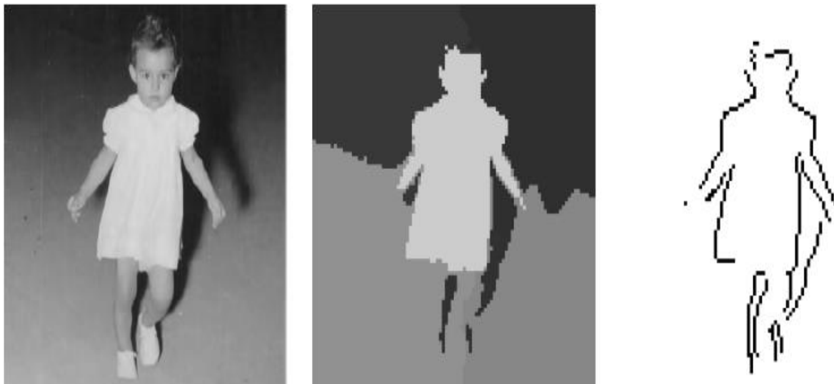
Figure 15 An original image, its segmentation and its edge map [82].
