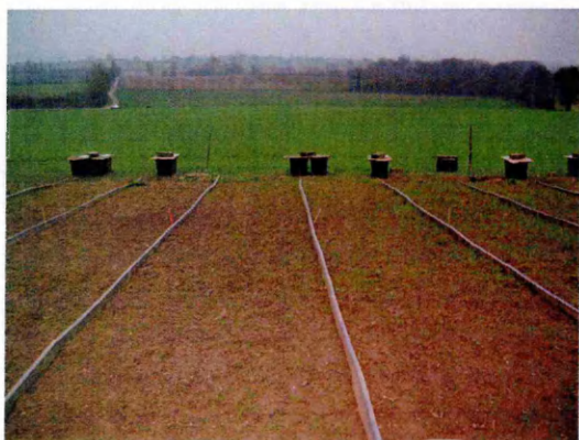
Plate 3.5. Hydrologically-isolated field plots were used to monitor sediment and P mobilisation at (a) the Rosemaund Holbach plots and (b) the Avon demonstration sites.
