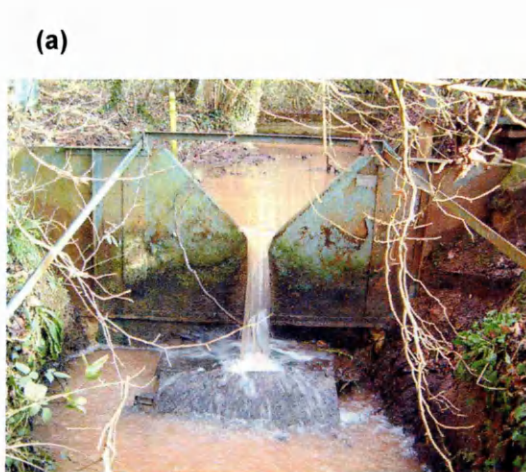
Plate 3.6. Flow was continuously monitored over (a) a thin-plate weir at the Jubilee station at Rosemaund and (b) through a purpose-built control section at the RD3 station at Redesdale.
