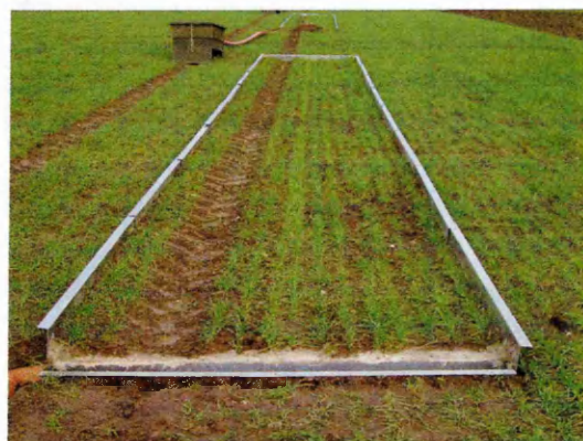
Plate 3.5. Hydrologically-isolated field plots were used to monitor sediment and P mobilisation at (a) the Rosemaund Holbach plots and (b) the Avon demonstration sites.
