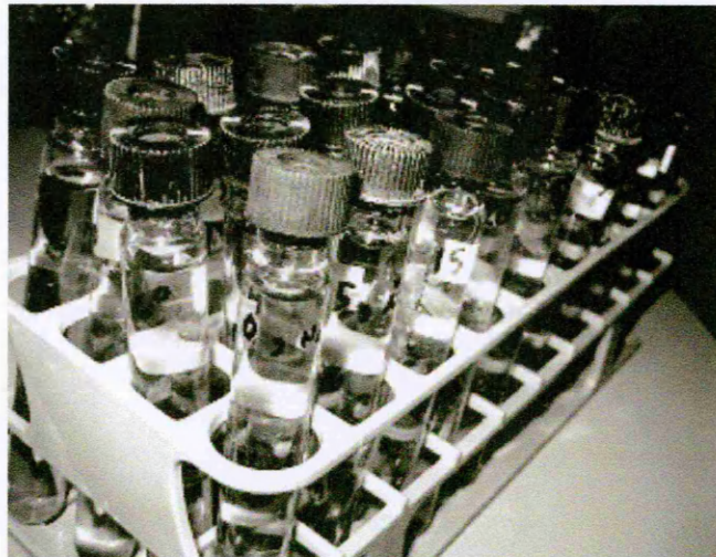
Figure 23 - Hungate tubes with rubber stoppers used for culturing experiments.
