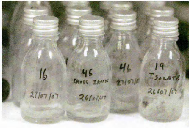
Figure 22 - Silver capped anaerobic bottles used for culturing experiments.
