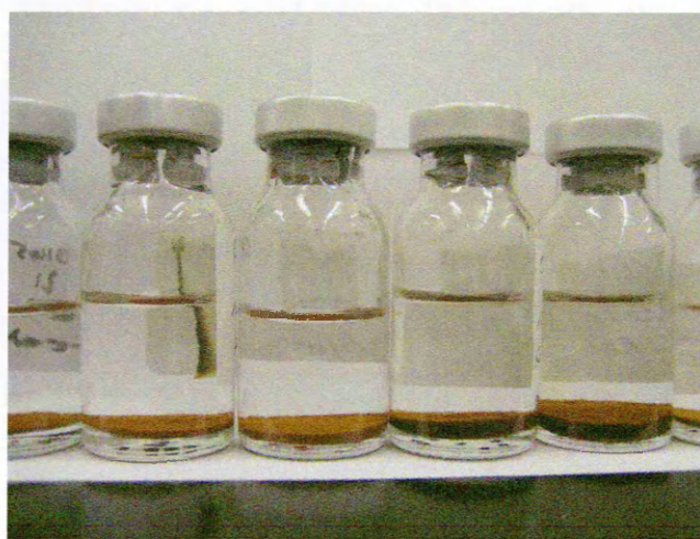
Figure 29 - USGS Fe Media showing colour change that indicates possible growth of cultures. Two bottles (right) contain darker iron precipitates, which was used as indication that these cultures warranted further examination.
