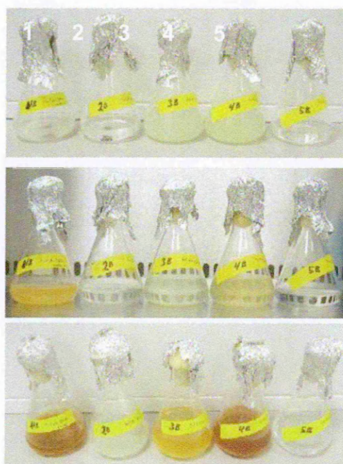
Figure 100 - Formation of precipitates during incubations period. (1) Solution A + Meteorite + T. ferrooxidans . (2) Solution A + Meteorite. (3) Solution A + Solution B (4) Solution A + Solution B + T. ferrooxidans . (5) Solution A + T. ferrooxidans .
