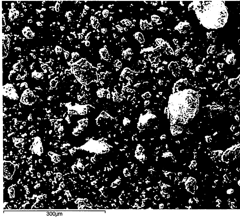
Figure 12: Secondary electron image of powdered bulk Murchison from which grain size distribution was ascertained (20 kV electron volatage, 1.2 nA beam current)
