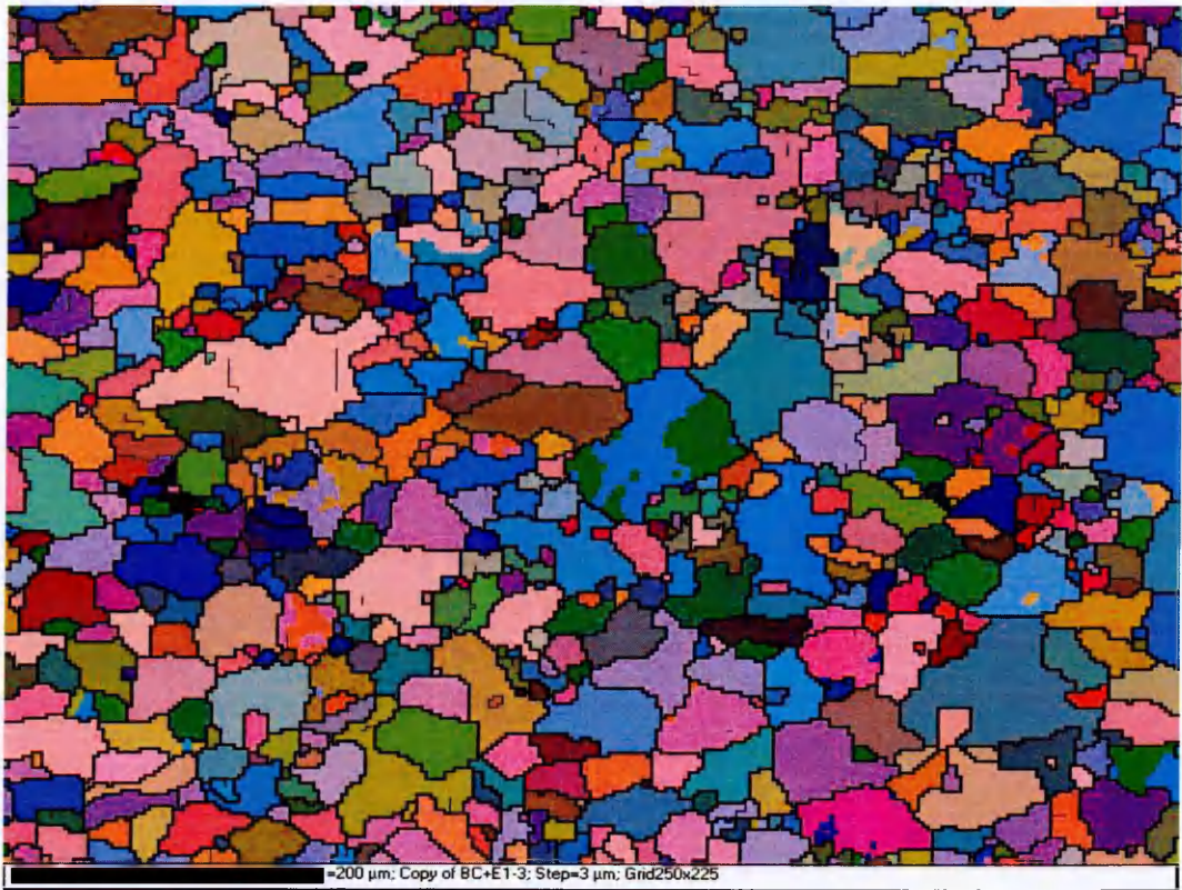
Fig. 3.3 - Grain size determination from (a) Optical microscopy (b) EBSD.
