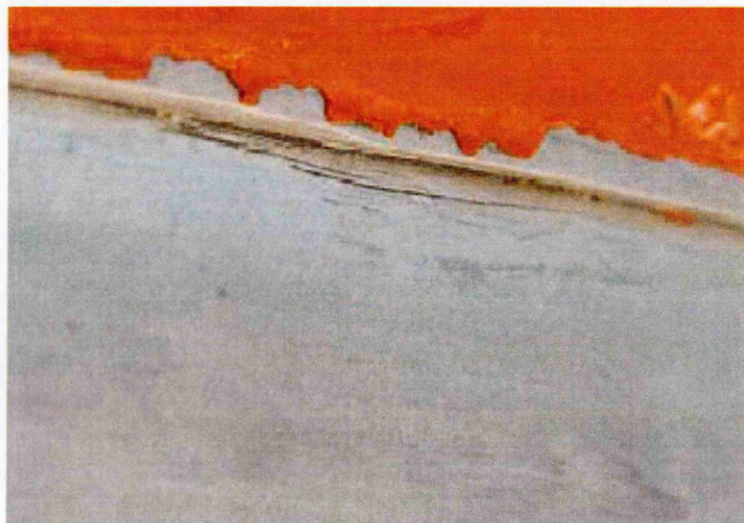
Fig. 2.1 - Scribe mark on a fuselage [29]
