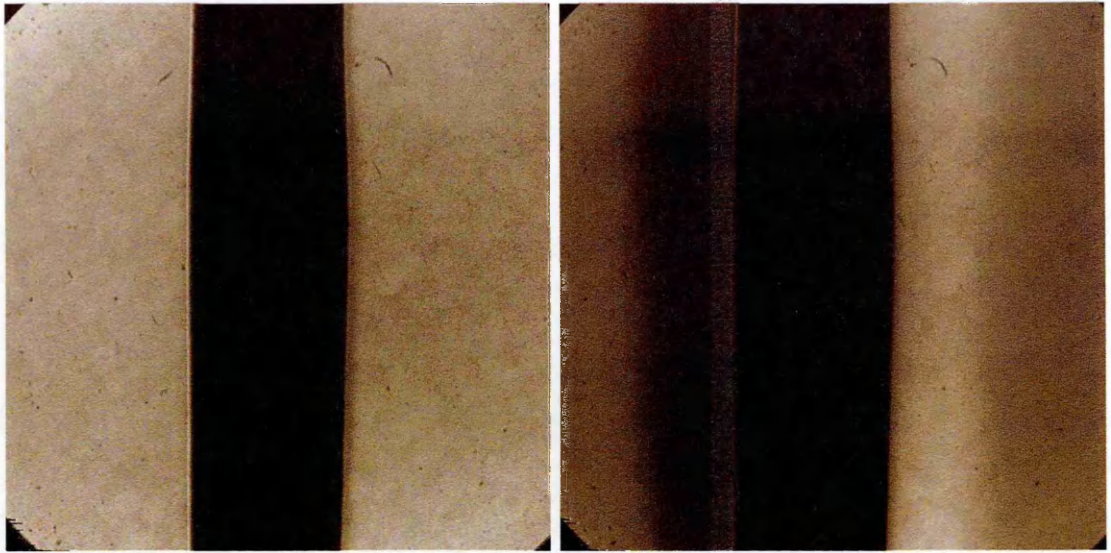
Figure 5.16: A schlieren image of the resistor pre-heating (left) and in steady state heating (right).
