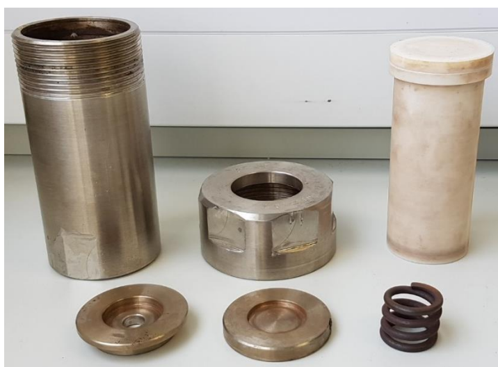
Figure 3.1. A standard autoclave showing the steel autoclave unit (1), steel autoclave screw-on lid (2), Teflon liner with lid (3), outer disc (4), inner disc (5) and spring (6).
