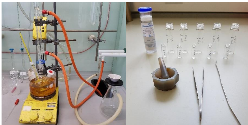
Figure 4.1. LEFT – experimental set-up of the reaction flask and filtration apparatus including Buchner flask, funnel and ring; RIGHT – Prepared labelled glass vials and pestle and mortar.
