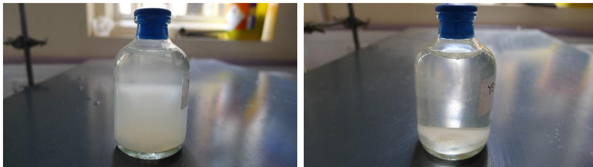
Figure 3.1: Thick gelatinous layer was observed immediately after the addition of \text{Na}_2\text{CO}_3 in the abiotic experiment without yeast extract (left). Over time, the gelatinous layer gets thinner and eventually vanished after 24-hour incubation (right). A longer period is required for the thinning process in the sample with high Mg/Ca and yeast extract and vice versa.
