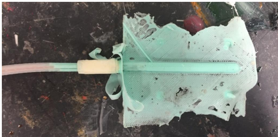
Figure 5.8: Casting Trial Of Flexible Bougie Tip Utilising Green Silicone (Shore Hardness 20)
