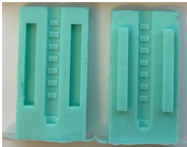
Figure 6.33: Steerable Tip Insert Development Iteration 5 Silicone Mould
