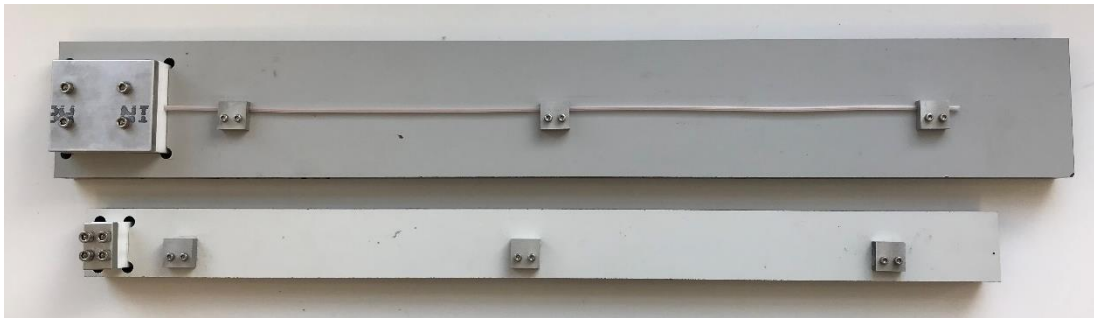
Figure 5.14: Manufactured Moulds & Supporting Structure
