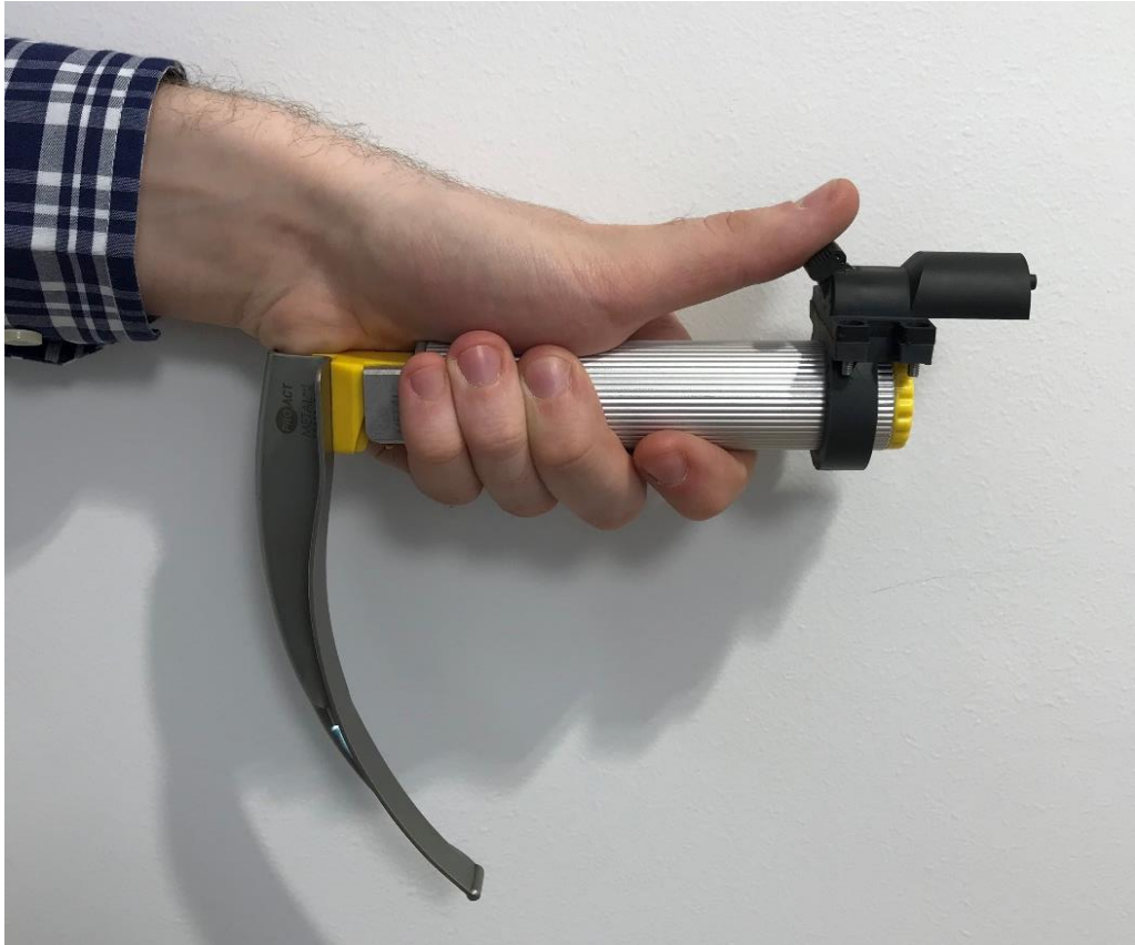
Figure 5.5: Manufactured Form Model Of The Control Adaptor Attached To A Proact Laryngoscope.
