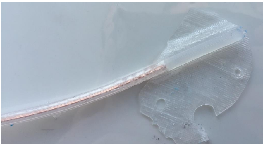
Figure 5.9: Flexible Tip Cast Out Of Medical Grade Silicone
