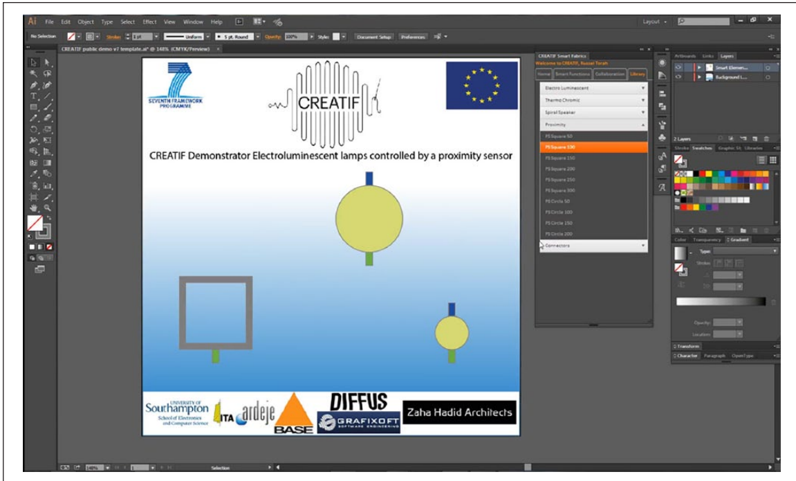
Figure 1. Example drawing and functional elements used in the design tool via the design tool add-on for Adobe Illustrator. The square represents the proximity or touch sensor. The circles represent the electroluminescent lamps.
