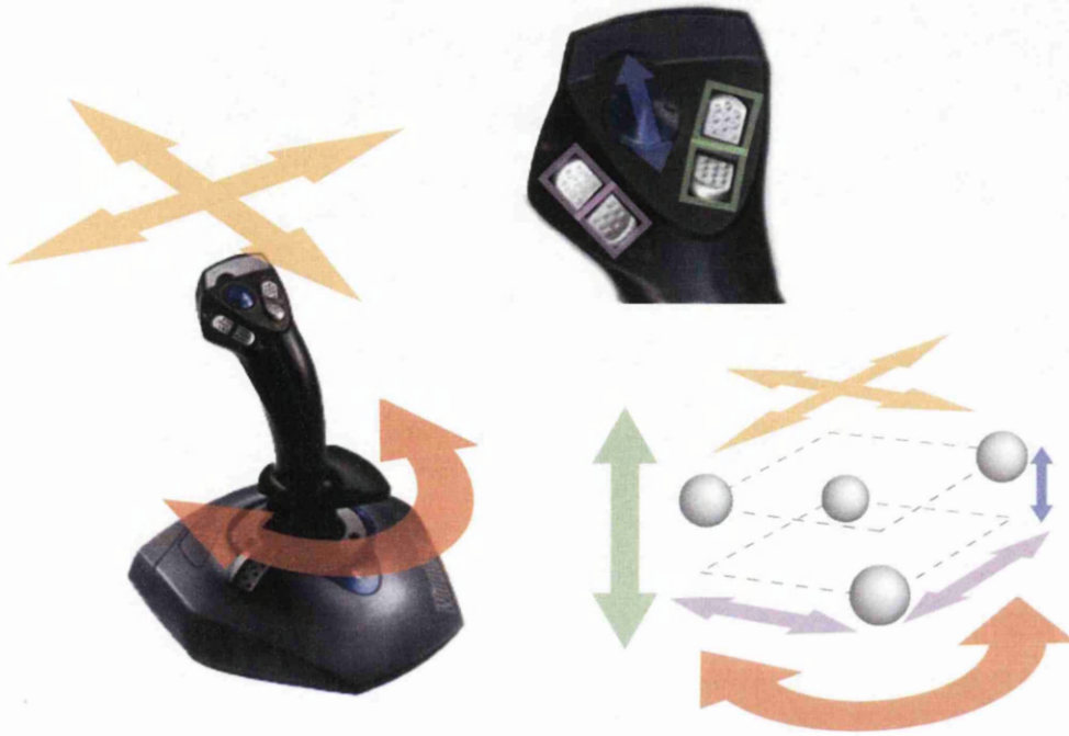
Figure 8.5: Representation of the degrees of freedom used by the joystick interface and the manipulation used by each. The xy position of the joystick represents the velocity of the centre of the four traps, the twist of the joystick relative to the base gives rise to a rotation of the square pattern with the speed of rotation being proportional to the angle of twist. Two buttons on the top of the joystick controls the size of the square in the xy plane and another four buttons on the base control the z height and the height difference between the sets of spots \delta z .
