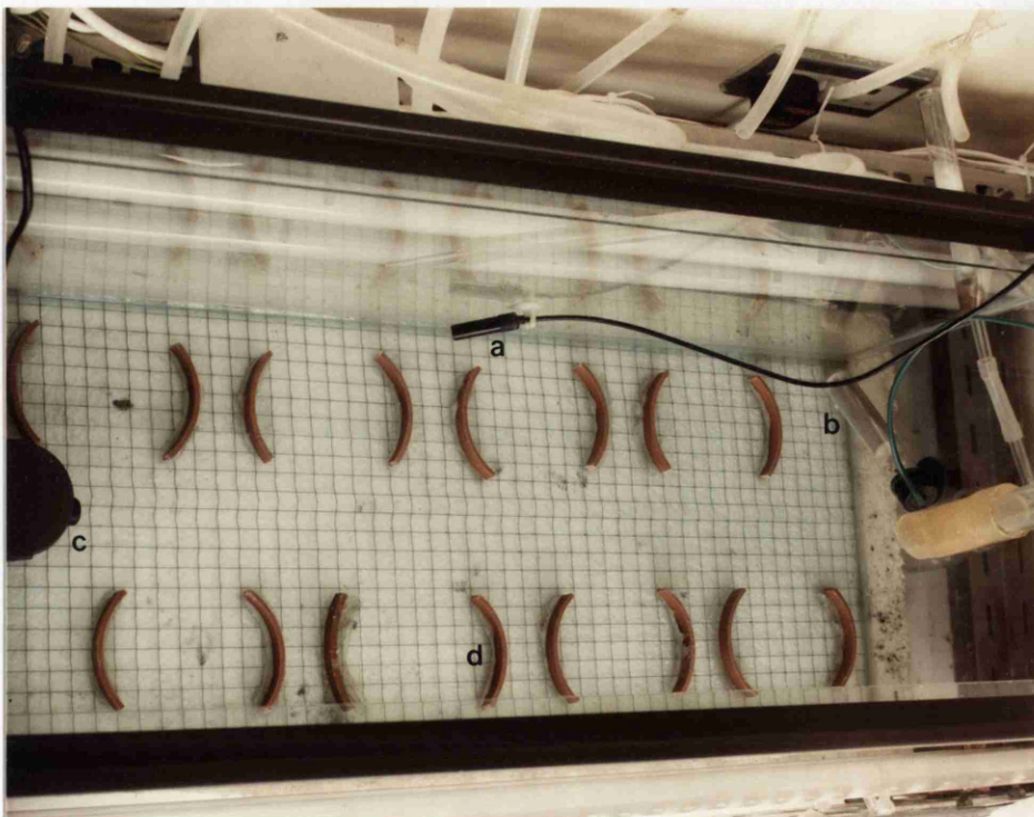
Plate 2: Batch Culture System: Top View (Empty) (a) temperature sensor (b) heater (c) mixer (d) staggered bottle holders
