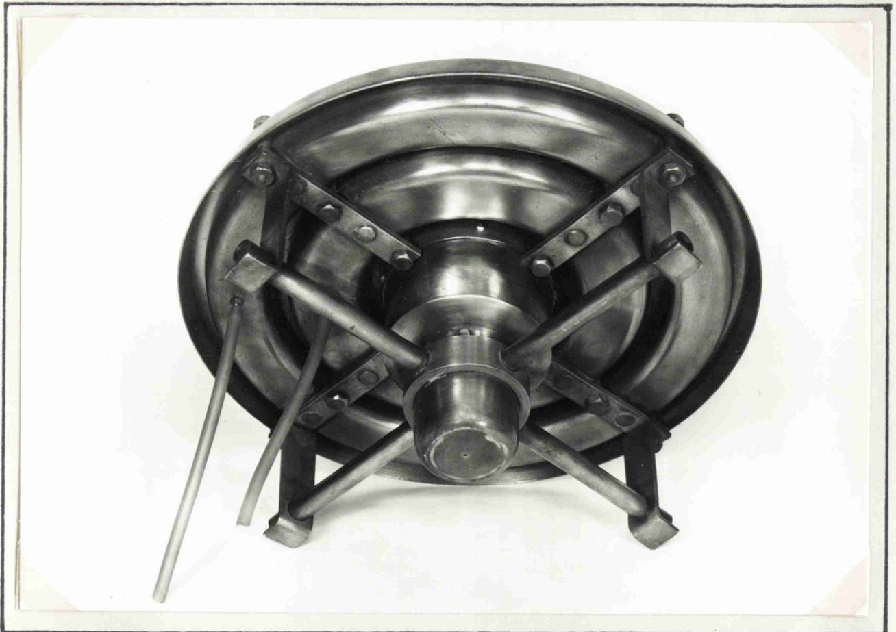
THE 12 INCH DIAMETER KUHNPLATE , THE LOWER VIEW SHOWING THE LIQUID DISTRIBUTERS AND THE CLEAR LIQUID HEIGHT MANOMETER TAPPINGS.
