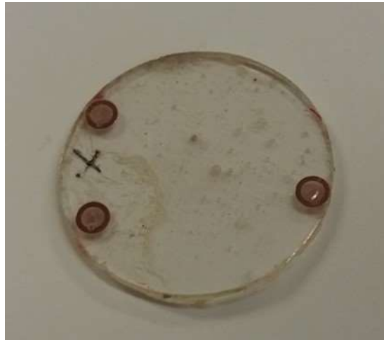
Figure 11: Completed grain mount. Polished and grain mount for SA10. The copper disks visible are labelled A, B, and C. Each disk includes a grid with the respective letter at the centre, and a larger letter on the rim. The letters and grids can be used to orient the grain mount and were used as reference points when producing spot coordinates for analysis.
