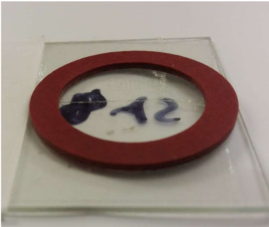
Figure 10: Grain mount preparation. In preparation for grain mounting double-sided adhesive tape was applied to a glass slide. The adhesive tape serves a dual purpose; firstly it allows the washer to be attached to the slide to contain resin later in the preparation of the sample mount. Secondly, the adhesive tape allows picked grains to be arranged in an ordered grid without risk of any grain becoming dislodged or loose. Grains in this sample are small; however the grid can be made out within the far portion of the washer.
