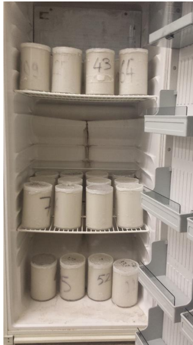
Figure 3-12: Curing specimens at low temperature.
