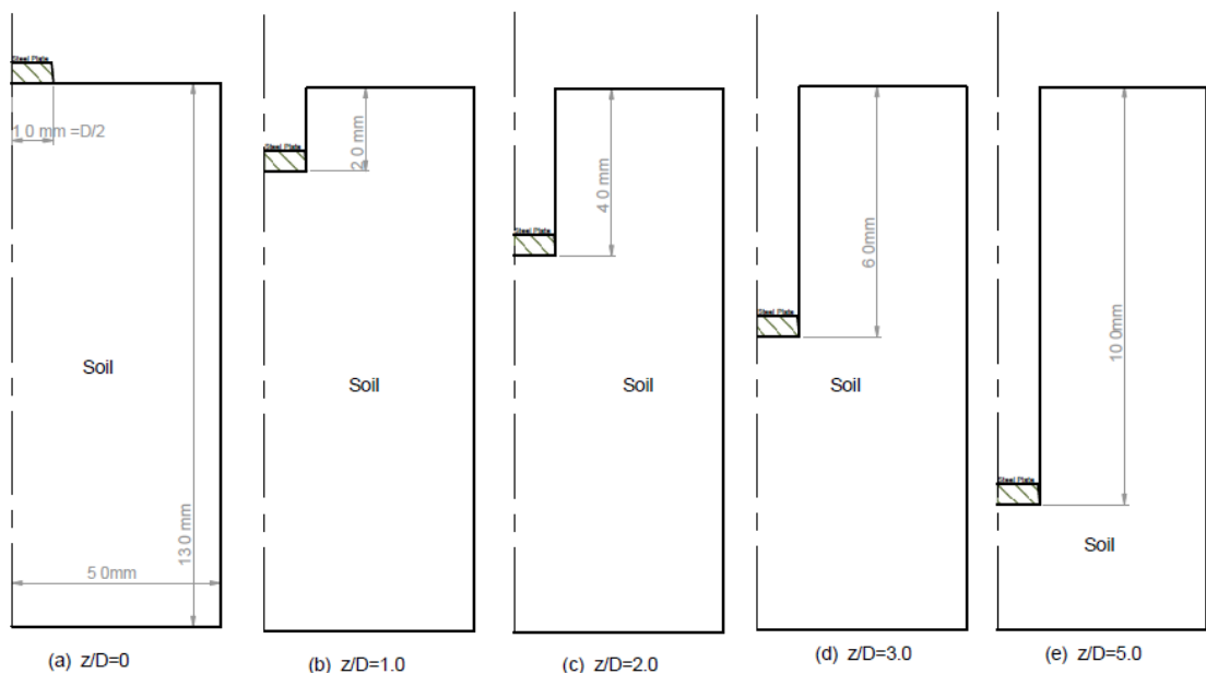
Figure 4-14: Geometric modelling of penetration by 20mm disc
