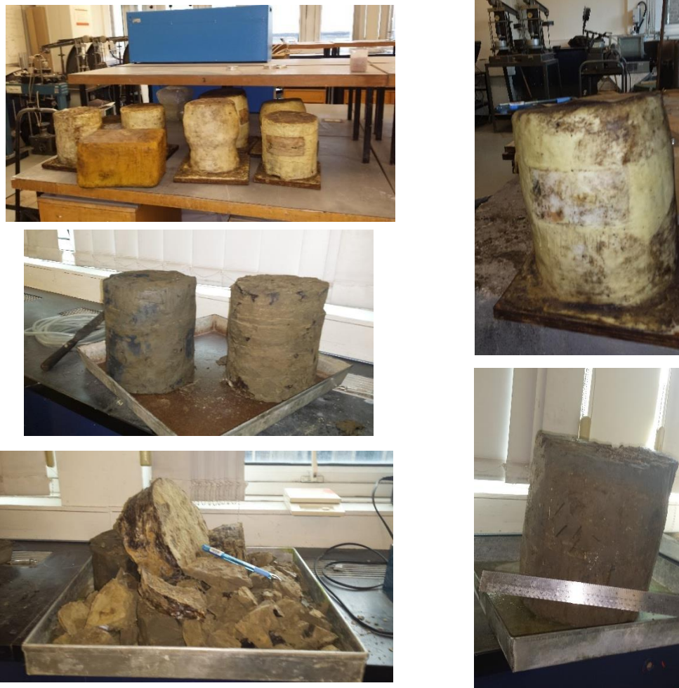
Figure 3-6: Grangemouth soil before and after de-waxing and cutting.
