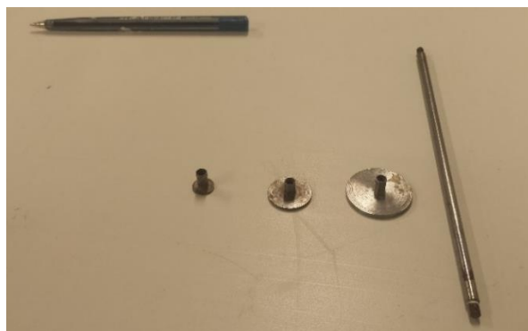
Figure 3-34: Penetrometer shaft and steel disc penetrometers.
