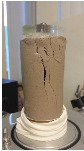
Figure 3-30: CB Bentonite specimen at failure in triaxial compression.
